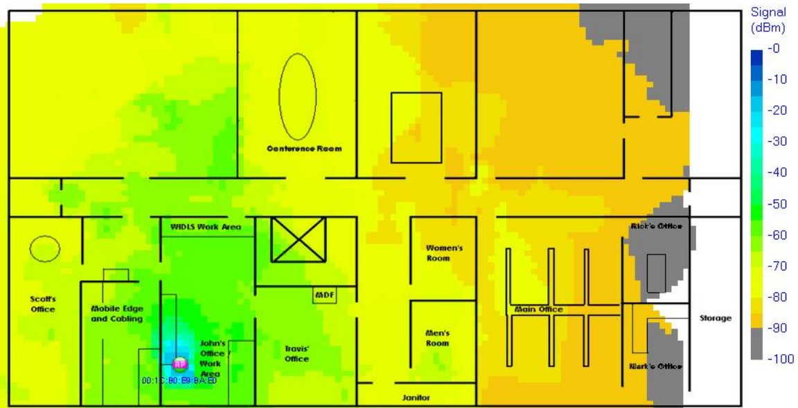
Fig. 2 1059-00 Site Survey Test with Cisco 1242 at 2 dBm Tx Power (August 18, 2010) 2.4 GHz with enclosure
